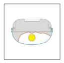
Parabolic flow recuperator for ASYMMETRIC direct distribution, for luminaires 160 mm wide. T8 - Flux recuperator in high-reflecting aluminium.
