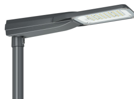
DigiStreet Mini - LED Module 4500 lm - 518 ClearStar WW - Safety class II - Distribution medium 11 - Dark gray - Luminaire surge protection level until 6 kV differential mode and 8 kV common mode - Spigot for diameter 62 mm
